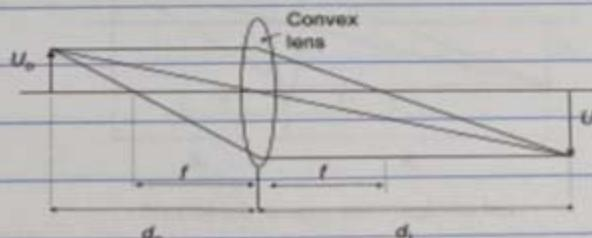
**FIGURE 1.5** Imaging with a single thin lens.
