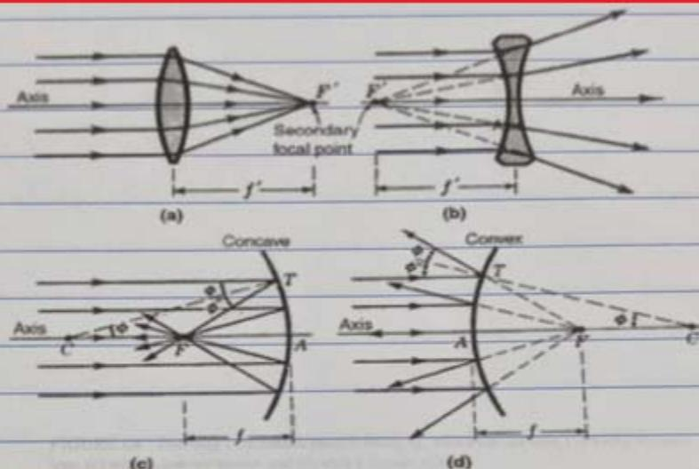
**FIGURE 1.4** Focusing a collimated parallel beam: (a) with a convex lens, (b) with a concave lens, (c) with a concave mirror, and (d) with a convex mirror.
